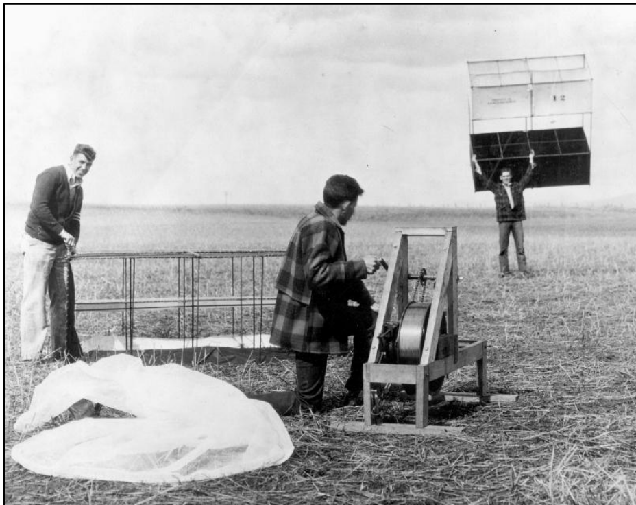
Fig. 7A. Tom Terrell (center) preparing to fly a weather bureau kite equipped with nets to study flight and dissemination of the mountain pine beetle in an area adjacent to lodgepole pine during an outbreak of the beetle. Only one bark beetle was caught; it was not a mountain pine beetle. Big Hole Basin, Montana.
