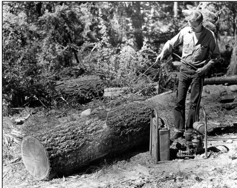
Fig. 16. A. Gasoline-motor-powered sprayer developed by Tom Terrell for applying insecticide formulations to kill bark beetle brood beneath bark of infested trees. It was designed originally with handles for carrying and operation by two people and consisted of a 2-cycle gasoline motor, a pump and a 5-gallon Jeep can containing the insecticide. Three million trees were sprayed with this equipment on the Targhee and Teton National Forests between 1957-1969. Direct control was abandoned when Amman & Baker (1972) showed that, treated or not, the residual stand ended up the same over time. Shown here is LeRoy Kline, using a pump borrowed from Terrell to test a formulation for preventing infestation of the Douglas-fir beetle in a felled tree. Kline was a summer assistant in 1959 on Mal Furniss' study in Idaho.
