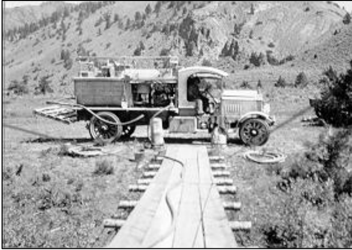
Fig. 19. In an attempt to control the spruce budworm in Cody Canyon, Wyoming, during 1930, a “high-power Fitzhenry Gupti sprayer” was used to apply 136,000 gals of spray containing 3864 lbs. of lead arsenate (Evenden 1931). The pump delivered 300 pounds of pressure through 1,500 feet of hose to a height of several hundred feet. Four or more crewmen were required to wrestle the lengthy hose, sometimes having to cross the Shoshone River to reach some of the summer homes and resorts.
