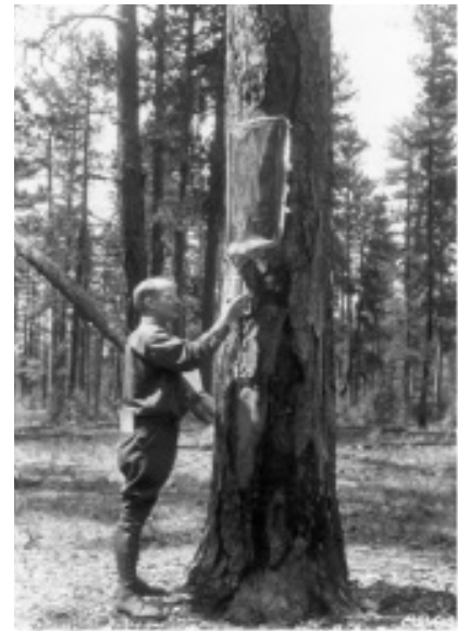
Walter Buckhorn and screen cage that he designed to trap western pine beetle brood that emerged from infested ponderosa pine, Prineville, OR, May 27, 1932. Variations of this cage were used subsequently by entomologists studying other bark beetles throughout the west. Photo PS no. 125, WFIWC archives. (Furniss 2000, Fig 11).
