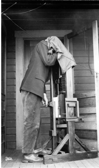
Camera stand constructed by J.E. Patterson for taking close-up photos of cone and seed insects being studied at Ashland, OR, 1915. Patterson had been an apprentice photographer before his employment at Ashland and later at the Palo Alto and Berkeley forest Insect Labs. This glass plate negative has been broken. Photo 2238 by J.E. Patterson, WFIWC archives. (Wickman et al. 2002, Fig. 2).
